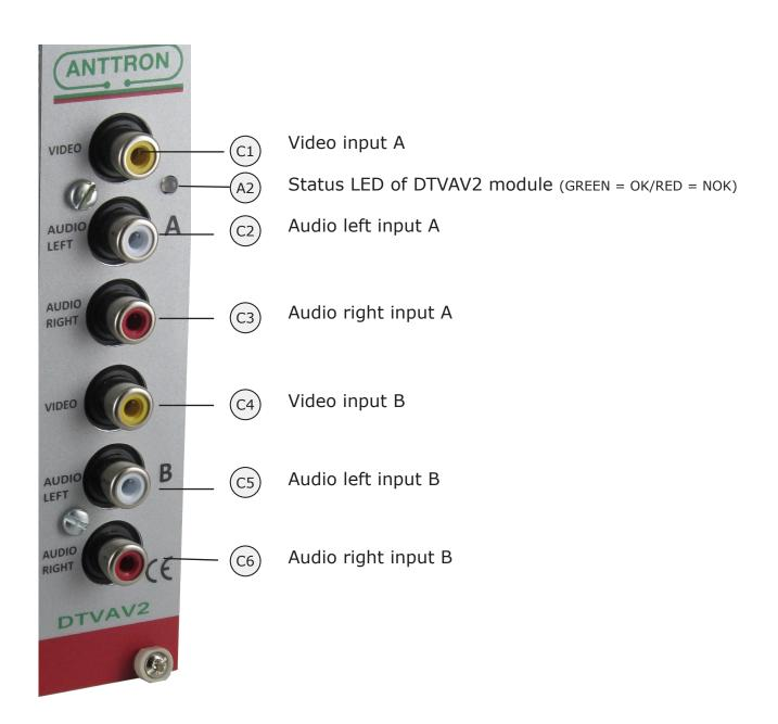
**DTVAV2**: this module performs the following function in the DTVRack
